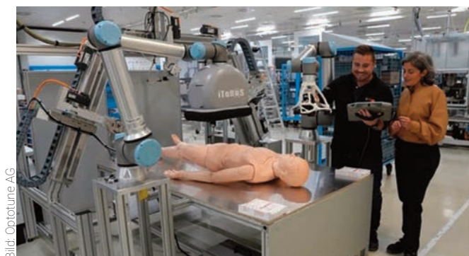
Figure 2 | Liquid lenses are used in early detection of potentially lethal skin condition. The Intelligent Total Body Scanner for Early Detection of Melanoma (iToBoS) project is developing an AI-powered diagnostic platform using high-resolution cameras equipped with liquid lenses.
