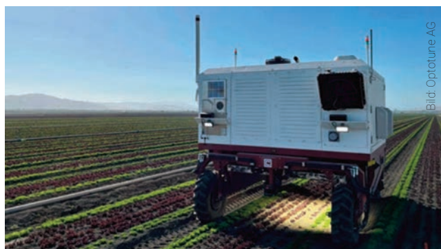
Figure 3 | Autonomous vehicle moves through a field, while scanning the surface below for weeds that are lased with 3mm accuracy using CO2 lasers equipped with liquid lenses.
